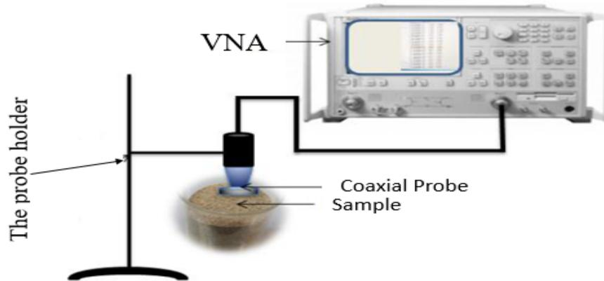
Figure 2: Experimental set up for Dielectric measurement
