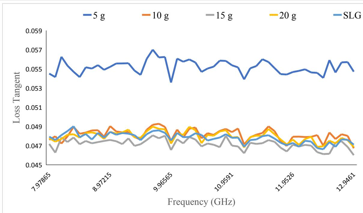
**Figure 5: Comparison of loss tangent for Different ratios of SLG/PCL Composites**
