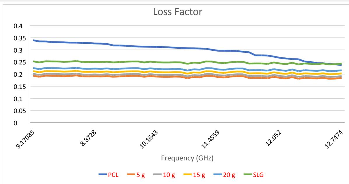
**Figure 4: Comparison of loss factor for Different ratios of SLG/PCL Composites**
