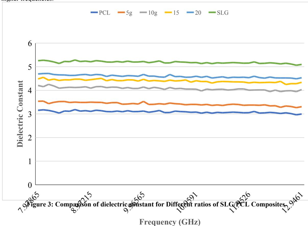
Figure 3: Comparison of dielectric constant for Different ratios of SLG/PCL Composites
