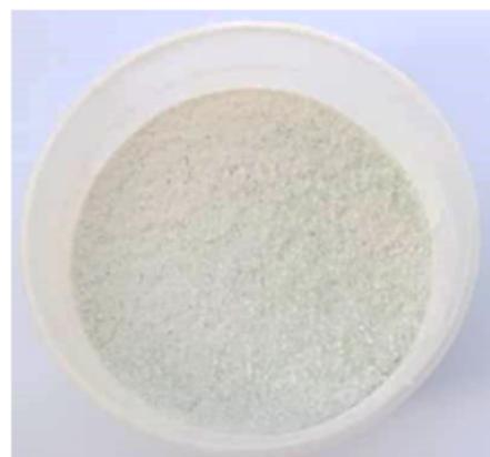
Figure1: Grinded Sodium Lime Glass
